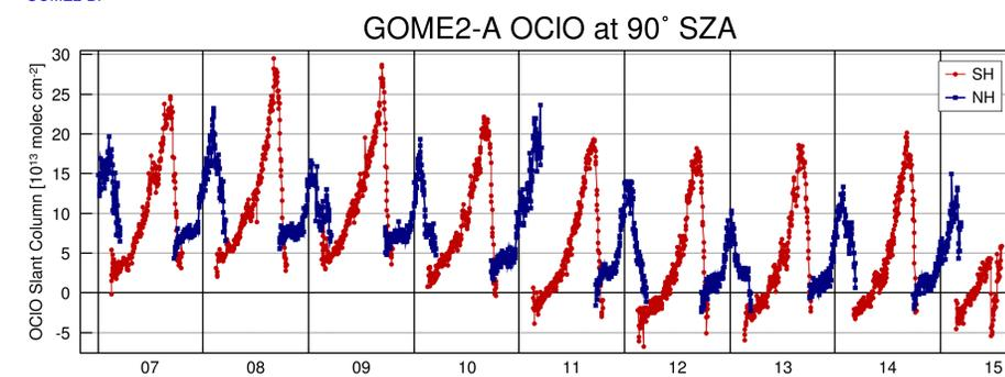
Figure 5 (top): GOME2-A OCIO at 90° SZA for both hemispheres. As the latitude at which SZA 90° is reached changes with season, the values are not over a constant latitude. No normalisation has been applied and a clear long-term drift is apparent.
