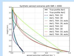
Fig. 2: Synthetic aerosol profiles and retrieved profiles for different parameters with and without a-priori scaling.
