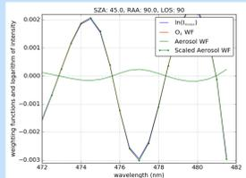
Fig. 1: Representation of the aerosol weighting function, which reproduces the spectral structures of the measurement and the  $O_4$  WF well.
