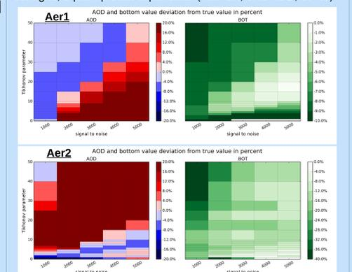
Fig. 3: Comparison of AOD (left) and bottom values (right) of retrieved profiles for different SNR and Tikhonov parameter values for aerosol scenarios without (top plots) and with prescaling of a-priori (bottom).
