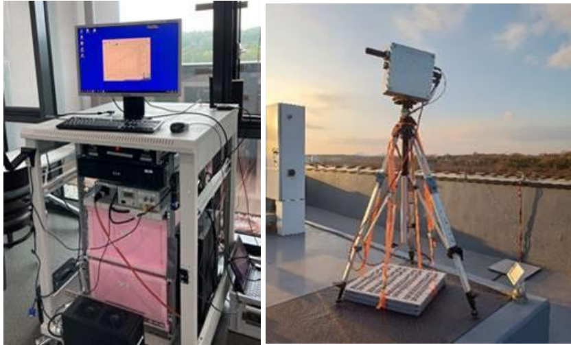
Figure 3.2.2: The MAX-DOAS telescope unit (right) as installed on the roof of the National Institute of Environmental Research (NIER) headquarters Incheon with coordinates (37.57°N, 126.64°E). On the left is the instrument and a computer to visualize the output data inside the building. (Photo by Andreas Richter, IUP)
